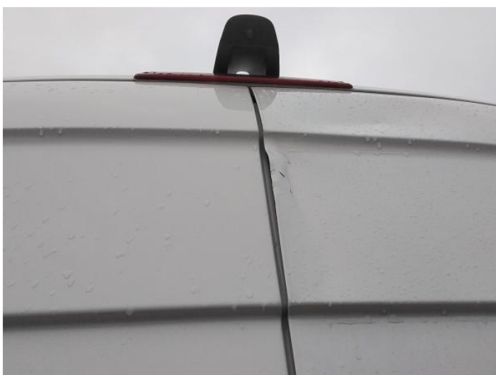
5: Door osr Dented With Paint Damage
