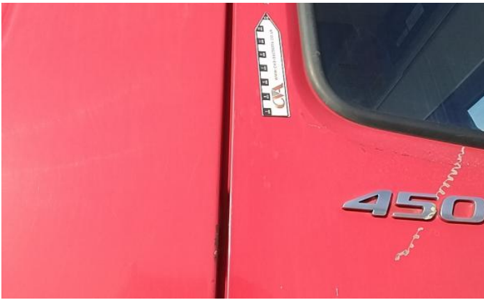
9: Wing Front Arch Extension os Scratched (Painted) Over 25mm Not Thru Paint
