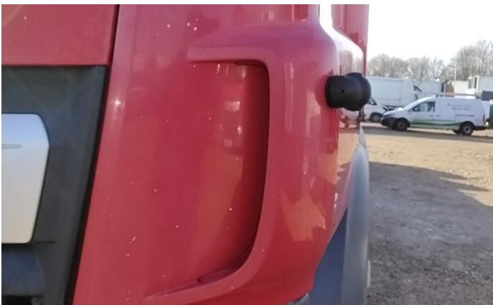
3: Bonnet Chipped Multiple Chips
